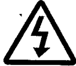
Warning, high voltage
