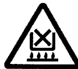
Caution, no road heating
